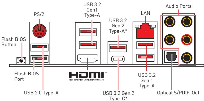
\*USB 3.2 Gen2 (3rd Gen AMD Ryzen™) or USB 3.2 Gen1 (2nd Gen AMD Ryzen™/Ryzen™ with Radeon™ Vega Graphics and 2nd Gen AMD Ryzen™ with Radeon™ Graphics)
