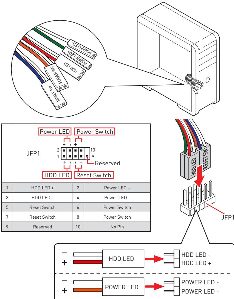
**Installing the Motherboard/ Installation des Motherboards/
