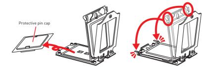
4. Close the load plate, and then turn the load plate screws clockwise a little with the AMD Torx screwdriver in the sequence  $1 \rightarrow 2 \rightarrow 3 \rightarrow 1 \rightarrow 2 \rightarrow 3$  until they are snug.
