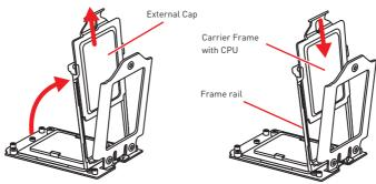
3. Remove the protective pin cap, and then close and buckle the frame rail.
