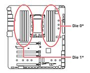
\* For 2990WX processor, DIMMC1, C2, D1 and D2 are controlled by Die1 and DIMMA1, A2, B1, B2 are controlled by DieO
