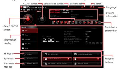
• GAME BOOST switch - click on the center button to switch GAME BOOST control between software (SW) and hardware (HW). The inner circle represents the current stage of hardware GAME BOOST and the outer circle stands for software. You can read the CPU frequency of each GAME BOOST stage by clicking on the ? icon at rightbottom corner.
