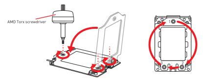
5. Tighten load plate screws until you hear a click from the AMD Torx screwdriver.
